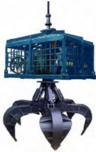
Figure 3.6: Example of a subsea grab tool (Source: DEME Group).
