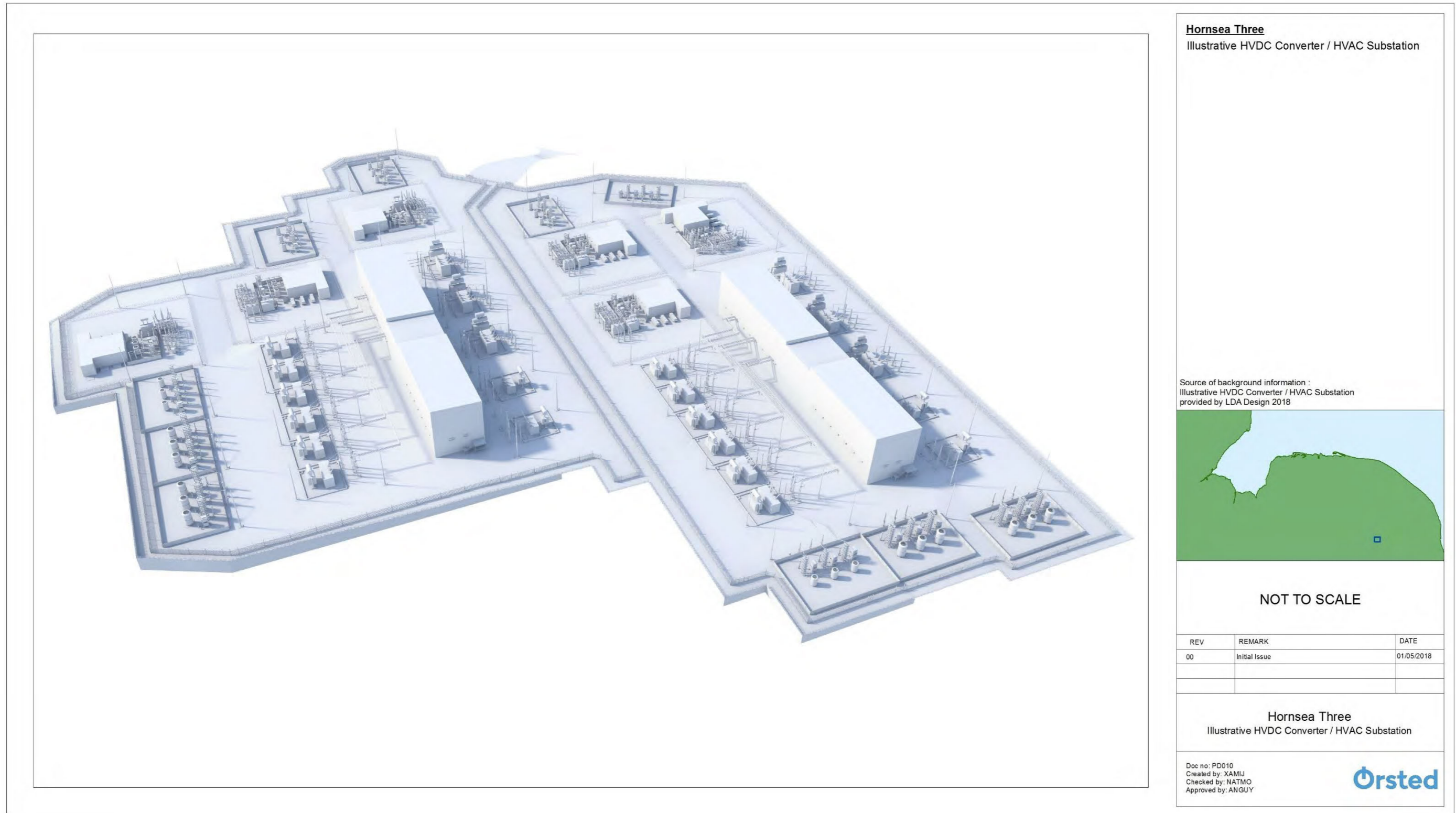
Figure 3.37: Indicative onshore HVDC converter/HVAC substation layout.
